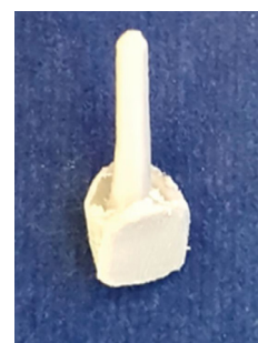
Post milling image of Post made from PEEK blocks ADVANTAGES
